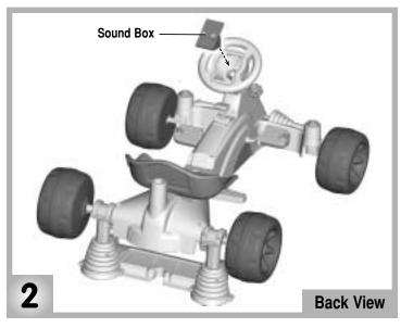
· Fit the sound box inside the center of the steering wheel.
