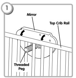
Fit the mirror onto the top crib rail so that the threaded peg extends out of the crib. Hold the mirror in place.
