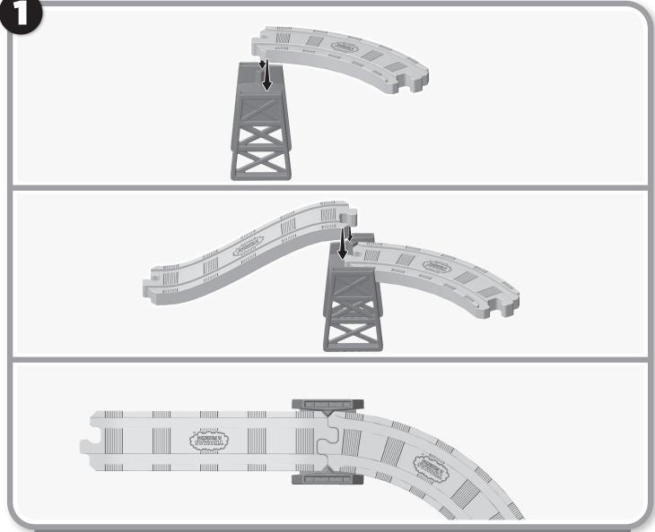
Place the end of one track piece on one side of the riser first and then place the second track piece on the riser as shown. Notches on the riser will fit between the two track pieces.
