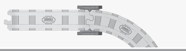
Place the end of one track piece on one side of the riser first and then place the second track piece on the riser as shown. Notches on the riser will fit between the two track pieces.
