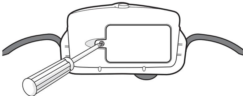
Loosen the screw in the battery compartment door and lift to remove the door.
