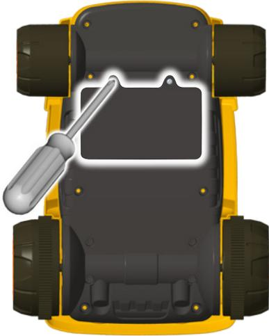
Loosen the screws in the battery door and remove the door. Insert four, new C (LR14) **alkaline** batteries.
