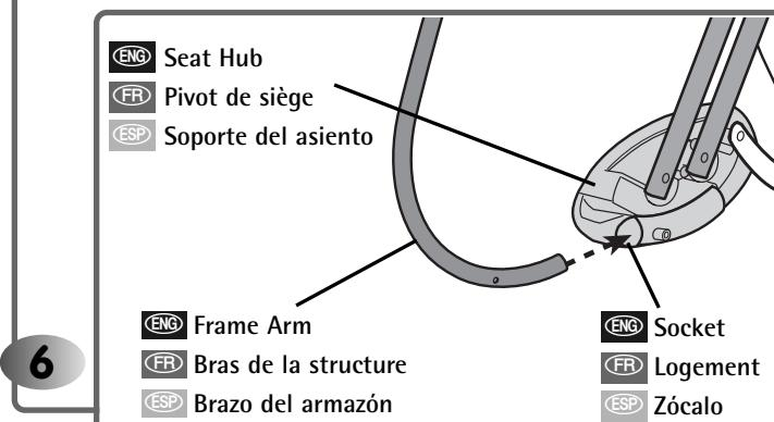
• Position the seat frame so that the tubes are upright, as shown.
