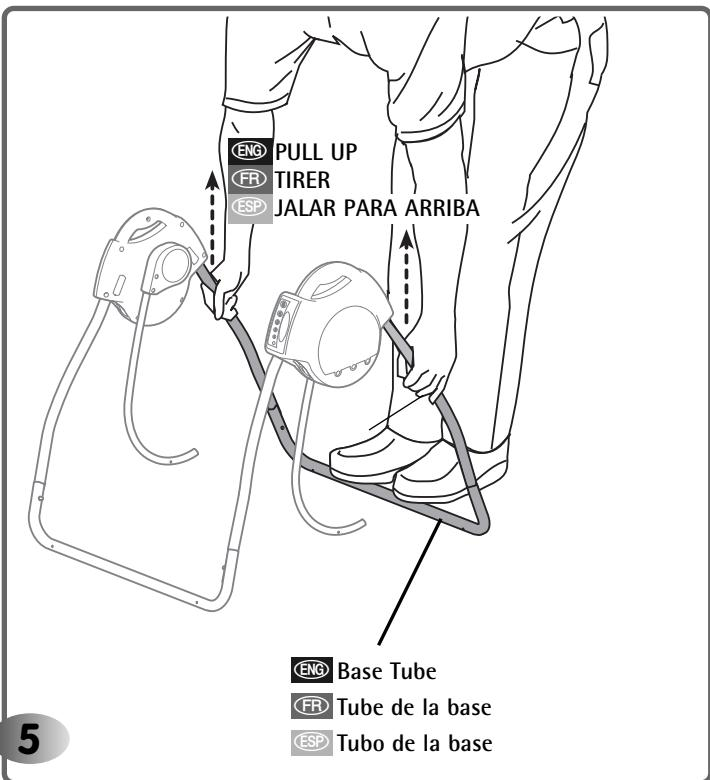
• While standing on the base tube, pull the back legs up. The back legs **should remain secured** to the base tube. If you can remove the back legs, you have not assembled them correctly to the base tube. Re-read and repeat assembly step 4.
