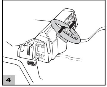
• Pull up on the steering wheel to be sure it is assembled correctly. If you can remove the steering wheel, you have not inserted the screw through both the bottom of the steering wheel and the steering column. Please review these instructions and re-assemble the steering wheel.
