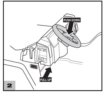
• While pulling up on the steering column, push down on the center of the steering wheel.
