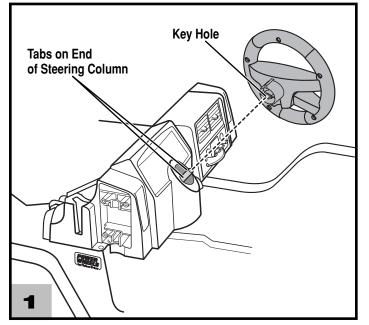
• Fit the keyhole inside the steering wheel to the tabs on the end of the steering column.
