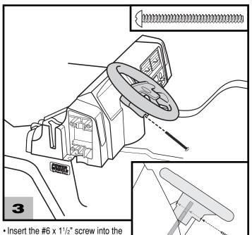
Insert the #6 x 1<sup>1</sup>/<sub>2</sub>" screw into the hole in the bottom of the steering wheel, through the hole in the
