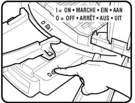
Move switches to OFF position before installing batteries.
