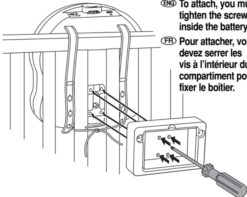
**(ENG)** To attach, you must tighten the screws inside the battery box.
