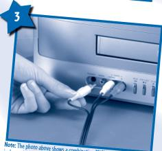
Note: The photo above shows a combination TV/VCR/DVD with input jacks on the front. Your TV or VCR may have input jacks on the back.
