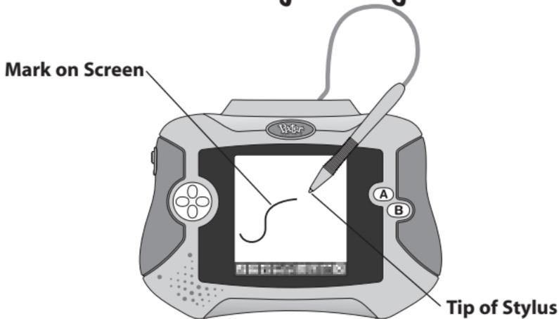
**IMPORTANT!** From time to time, the mark made on your screen from the stylus and the location of the tip of the stylus may not align. When this happens, you must calibrate the stylus.
