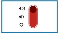
Locate the power-volume and mode switches on the side of the doorbell. Slide to turn power ON with low volume **4**), ON with high volume **4**)) or OFF **O**.
