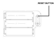
Helpful Hint: If your Eye-Lock Room Guard is not working correctly or you have forgotten your code, press the RESET button and reenter your Eye Code. If your Eye-Lock Room Guard is still not working correctly, you might need to change the batteries.
