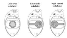
First place the Eye-Lock Room Guard over the door knob/handle to see how it will fit on your door. You will attach your Eye-Lock Room Guard to the door by placing it over the doorknob, using the special tape attached to the back. All you have to do is remove the paper backing from the special tape, allowing the adhesive to be exposed. Line the oval
