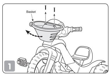
Loosen and remove the two screws in the basket.
