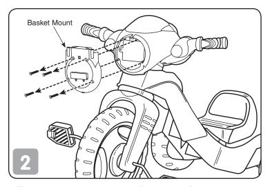
Then, loosen and remove the four screws from the basket mount. Remove the basket mount.
