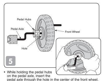
Push the pedal hubs into the center of the front wheel until they are flush with the surface of the front wheel.
