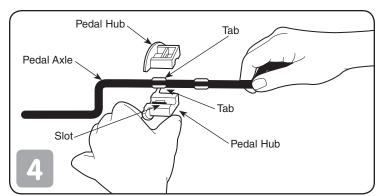
• Fit two pedal hubs onto the pedal axle tabs. Make sure the tabs fit into the slot in each pedal hub.
