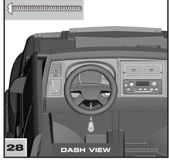
• Insert a #6 x 11/2" screw into the hole in the base of the steering wheel. Tighten the screw.
