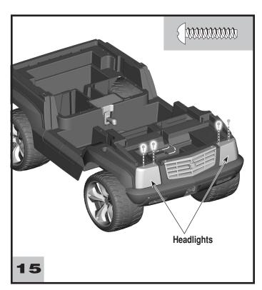
• Insert two #8 x <sup>3</sup>/4" screws into the top edge of each headlight. Tighten the screws.
