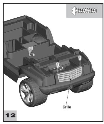
• Insert two #8 x 3/4" screws the top of the grille. Tighten the screws.
