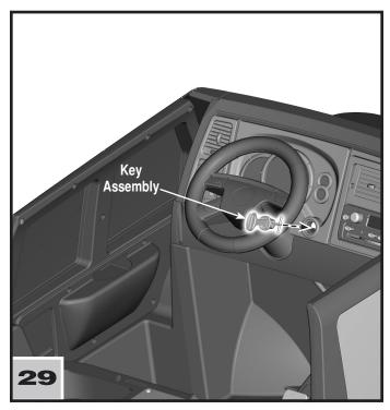
• Insert and "snap" the key assembly into the slot in the dash.
