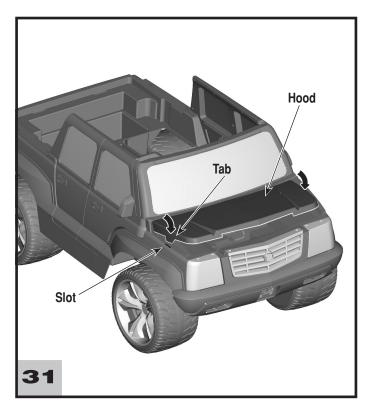
Lower and fit the side tabs on the hood into the slots on each side of the front end of the vehicle.
