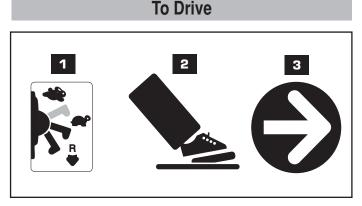
IMPORANT! To avoid damaging the motors and gears, stop the vehicle before shifting between low and high speed.
