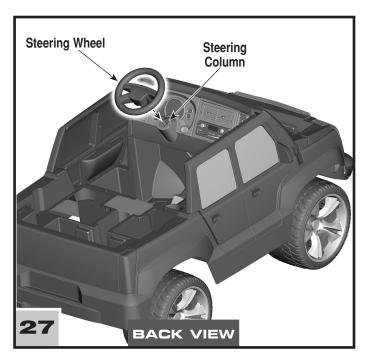
• While supporting the steering column in place, fit the steering wheel onto the end of the steering column.
