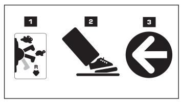
**IMPORTANT!** To avoid damaging the motors and gears, stop the vehicle before shifting from forward to reverse  $\clubsuit$ .
