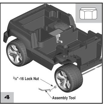
• Place a <sup>3</sup>/8" -16 lock nut (rounded side out) onto a front axle.
