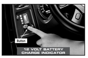
**IMPORTANT!** Do not press the 12 volt battery charge indicator while the vehicle is moving.
