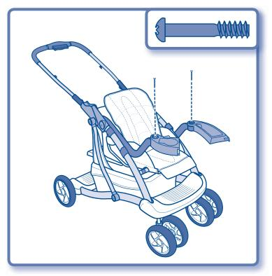
• For proper function, you must **fully** tighten the M5 x 1<sup>1</sup>/<sub>4</sub>" bolts in each armrest. Tighten these screws fully with a Phillips screwdriver.
