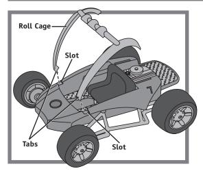
• Insert and "snap" the tabs on the front of the roll cage into the slots near the front of the dune buggy.
