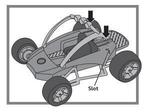
• Insert and "**snap**" the tabs on the back of the roll cage into the slots near the back of the dune buggy.
