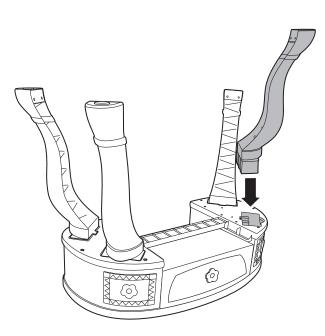
· Insert the assembled stool legs into the base as shown.
