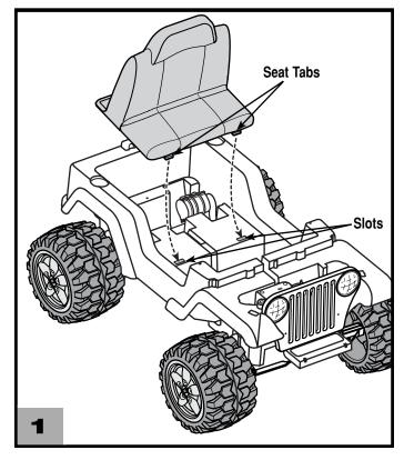
• Fit both tabs on the front end of the seat into the slots in the vehicle.
