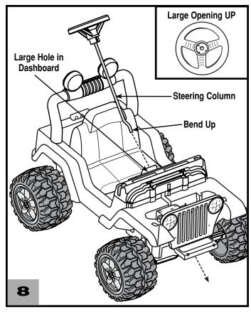
Insert the steering column (with steering wheel) into the large hole
