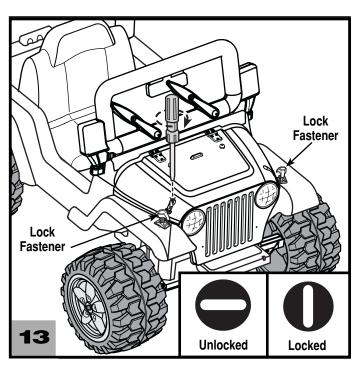
Using a slotted screwdriver, turn each lock fastener in the hood
