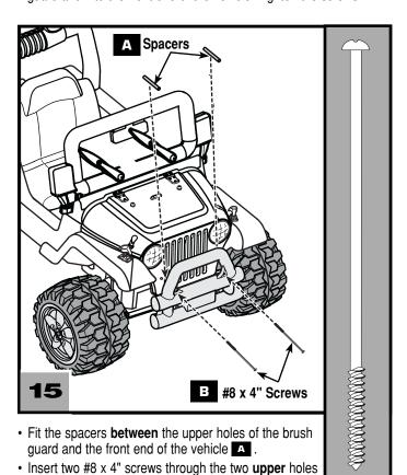
in the brush guard, through the spacers and into the front end of the vehicle **B** . Tighten the screws.
