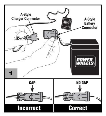
Plug the battery connector and charger connector together. Push firmly to make sure the two connectors are completely joined.
