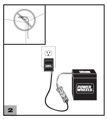
• Plug the charger into a standard 120 volt wall outlet.
