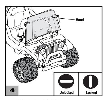
Lower the hood on the vehicle. Using a slotted screwdriver, turn each lock fastener ¹/₄ turn to the locked
