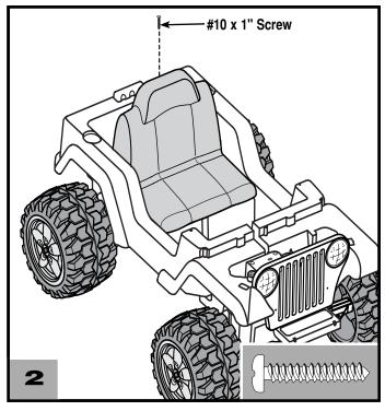
Insert a #10 x 1" screw into the back edge of the seat. Tighten the screw.
