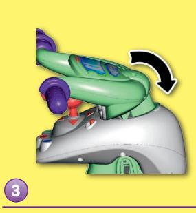
Next, push the handlebar forward and down in place.
