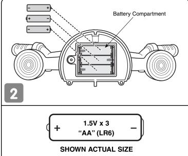
*Hint:* When sound or lights become faint or stop, it's time for an adult to replace the batteries. We recommend the use of **alkaline** batteries for longer battery life.
