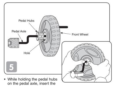
pedal axle through the hole in the center of the front wheel.Push the pedal hubs into the center of the front wheel until
