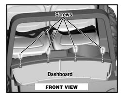
• We recommend the use of a short-shaft Phillips screwdriver to tighten the four screws in the dashboard.
