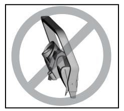
• The windshield is **not properly** assembled. Remove the windshield and turn it around so that it bends forward.
