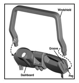
*Hint:*The windshield and dashboard are factory assembled and taped. If these parts come apart after removing the tape, follow this assembly step.
