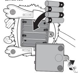
• Unscrew the battery cover with a Phillips-head screwdriver (not included). • Remove batteries included for demonstration purposes only and dispose of them safely.
