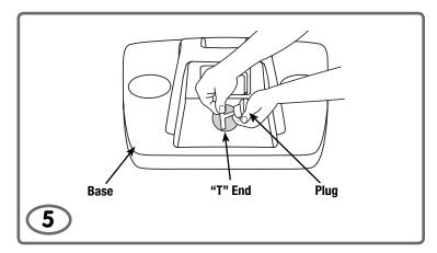
• Bend the "T" end of the plug and insert it into the hole in the base.
