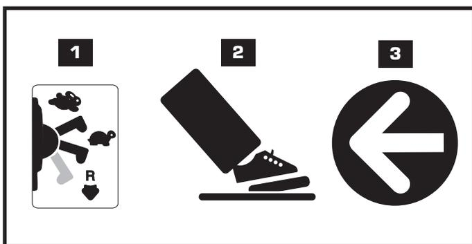
**IMPORTANT!** To avoid damaging the motors and gears, stop the vehicle before shifting from forward to reverse.
