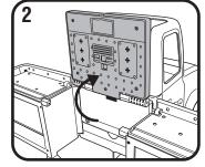
2. Hinge the flatbed of the truck upward this becomes the pegboard of the workbench.
