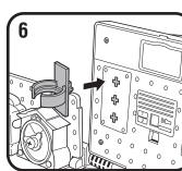
6. Insert the two tool clips into the main pegboard.
