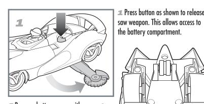
Remove battery cover with a Phillips head screwdriver (not included). Remove batteries included for demonstration purposes and dispose of them safely. Insert 3 new AG13 (LR44) button cell batteries in the orientation shown. Replace battery cover and tighten screw. For best performance use only alkaline batteries. Replace batteries if lights dim or do not function properly.
