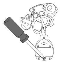
For best performance, we recommend replacing the batteries that came with this toy with two, new "AAA" (LR03) alkaline batteries.
