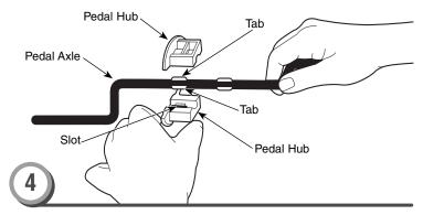
• Fit two pedal hubs onto the pedal axle tabs. Make sure the tabs fit into the slot in each pedal hub.
