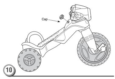
• Insert and "snap" the cap into the hole in the frame.
