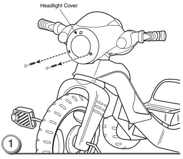
Loosen and remove both screws from the headlight cover.
