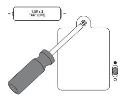
For best performance, we recommend replacing the batteries that came with this toy with three, new "AA" (LR6) alkaline batteries.
