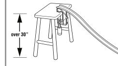
To regulate speed of car, change the height of the track. Higher clamp positions should produce higher speeds.
