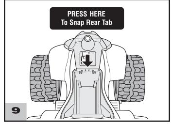
• Press firmly on the back of the cowling to snap the rear tab into the slot in the vehicle.
