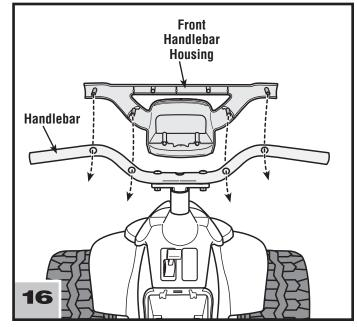
• Fit the front handlebar assembly into the front of the handlebar.
