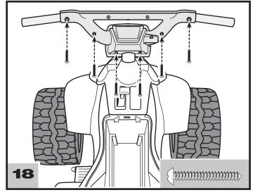
• Insert six #6 x 1" screws through the back handlebar assembly, as shown. Tighten the screws.
