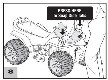
• Press firmly on each side of the cowling to snap the four side tabs into the slots in the vehicle. Make sure the rear tab stays aligned with the slot.
