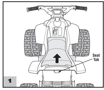
• Press the tab under the back of the seat and lift to remove the seat.
