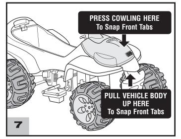
• Press firmly on the front of the cowling to snap the four, front tabs into the slots in the vehicle. Make sure the side and rear tabs stay aligned with the slots.
