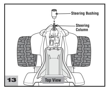
**Hint:** You may want the help of another adult to support the steering column near the steering linkage while assembling the handlebar to the vehicle.
