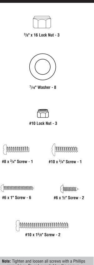
**Note:** Tighten and loosen all screws with a Phillips screwdriver. Do not over-tighten the screws.
