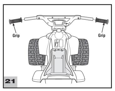
Fit a grip onto each end of the handlebar. If it is difficult to slide the grips onto the handlebar, moisten the grips with warm water first.
