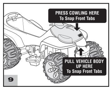
Press firmly on the front of the cowling to snap the four, front tabs into the slots in the vehicle. Make sure the side and rear tabs stay aligned with the slots.
