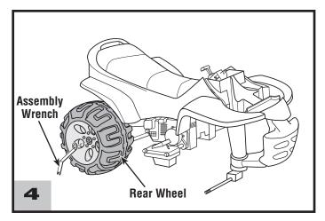
• Completely tighten the lock nut on the rear wheel assembly with the assembly wrenches.
