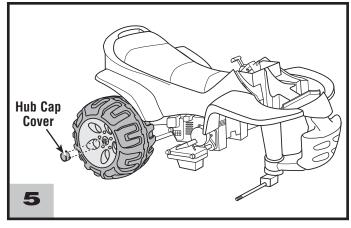
• Fit a hub cap cover onto each rear wheel and push to "snap" in place.
