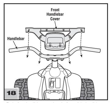
• Fit the front handlebar cover into the front of the handlebar.
