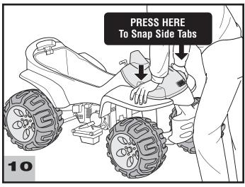
Press firmly on each side of the cowling to snap the four side tabs into the slots in the vehicle. Make sure the rear tab stays aligned with the slot.
