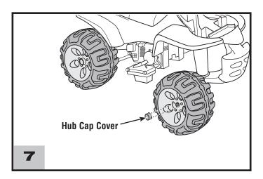
• Fit a hub cap cover onto each front wheel and push to "snap" in place.
