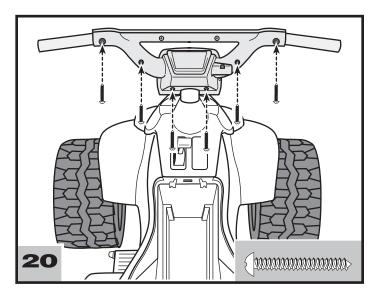
• Insert six #6 x 1" screws into the handlebar assembly, as shown. Tighten the screws.
