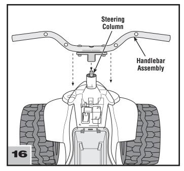
**Hint:** You may want the help of another adult to support the steering column near the steering linkage while assembling the handlebar to the vehicle.
