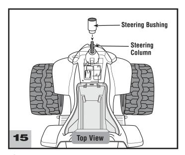
• Slide the steering bushing, narrow side down, onto the steering column and into the vehicle neck.
