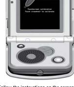
To calibrate the stylus to the touch screen, insert the tip of the stylus into the Calibration Hole → on the back of iXL™.  Follow the instructions on the screen and touch each mark with the stylus. Press any button when you are finished to exit the calibration screen
