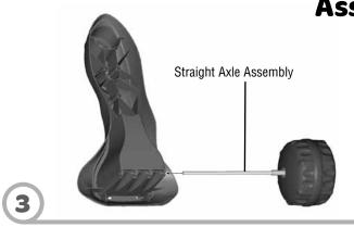
Turn the frame upside down. Insert the straight axle assembly through the holes in the rear of the frame.
