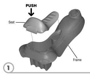
Fit the seat onto the frame. Push firmly near the back end of the seat to "snap" it into place.
