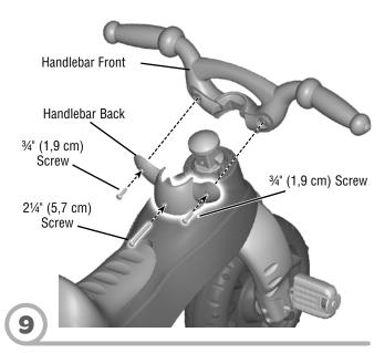
• Fit the handlebar front to the fork post.
