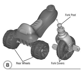
• With the fork covers facing the rear wheels, insert the fork post up through the hole in the neck of the frame.
