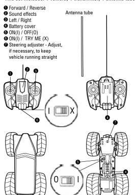
Insert loose antenna wire into antenna tube and secure by pushing it firmly into the hole in the transmitter.
