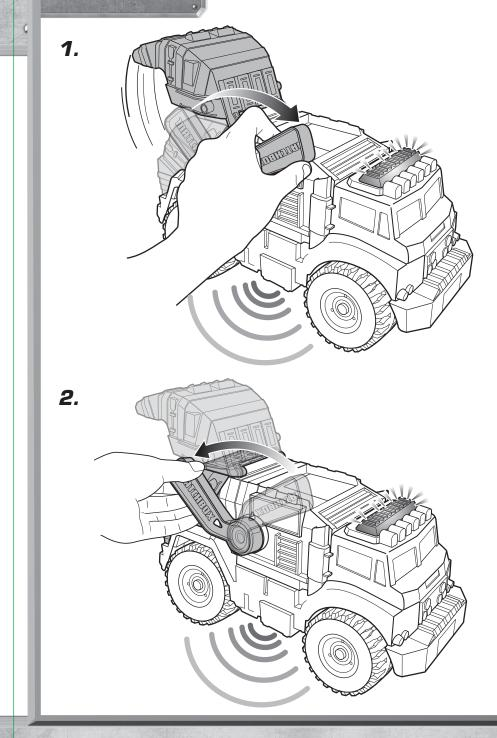
of them safely. To replace batteries, use a Phillips head screwdriver (not included) to open the battery cover. Remove and set aside. Install 3 new button cell (AG13, LR44) batteries as shown. Replace battery cover and tighten screw. For longer life use alkaline batteries. When exposed to an electrostatic source, the product may malfunction. To resume normal operation, remove and re-install the batteries.
