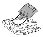
• Fit the tabs on the rechargeable battery pack into the slots in the battery compartment.
