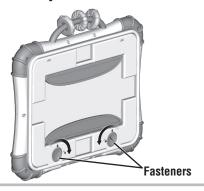
• Using a coin, turn each fastener to the unlock ∩ position.
