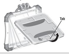
• Grasp the tab on the door and lift to remove the door.
