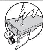
Push fingers through holes on bottom to remove batteries.
