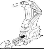
9. Use tool to remove excess wax.
