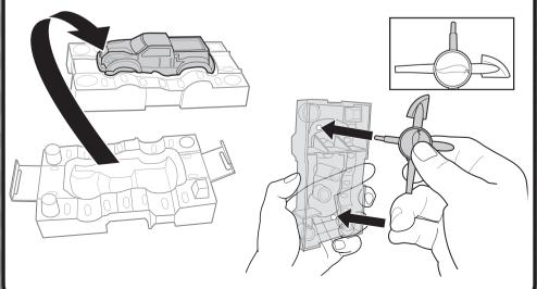
Carefully pry and lift the car body with the tool to loosen it further.
