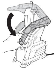
7. When cooldown cycle is complete, the door will unlock. Pull door open.
