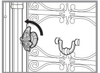
Turn counter-clockwise to secure latch.
