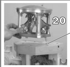
Thread cord through hole. Snap columns into roof.
