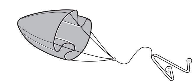
Open trap and put chute and string with "V" turned up in trap as shown. Close trap door.
