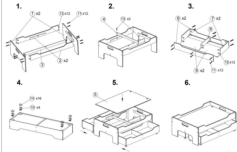
WHEN ASSEMBLING THIS ITEM, YOU MUST TIGHTEN ALL SCREWS SIMULTANEOUSLY. DO NOT TIGHTEN ANY SINGLE SCREW COMPLETELY AS THIS MAY CAUSE THE ITEM TO BECOME OUT OF ALIGNMENT. IF THIS HAPPENS, IT WILL REQUIRE YOU TO LOOSEN ALL THE SCREWS AND BEGIN AGAIN BY TIGHTENING ALL SCREWS SIMULTANEOUSLY. ADULT ASSEMBLY REQUIRED.PHILIP'S SCREW DRIVER IS NOT PROVIDED.
