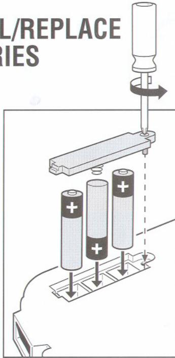
Remove battery cover with a Phillips screwdriver (not included) and set aside. Insert three "AA" alkaline batteries (not included) as shown and replace battery cover.
