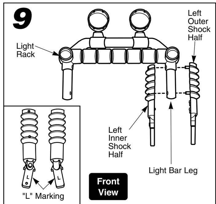
**Note:** The shock set halves and the light bar legs are marked "L" and "R".
