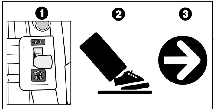
**Note: To avoid damaging the motors and gears, make sure to stop the vehicle before switching from forward to reverse .**
