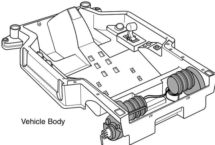
**\*IMPORTANT!** The front axles have been placed in the vehicle body motors for shipment. Please remove the front axles from the motors.
