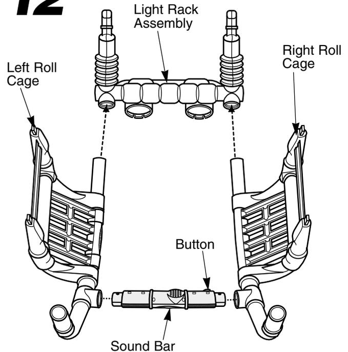
**Hint:** It is easiest to assemble the roll cage by positioning the parts upside down as shown.
