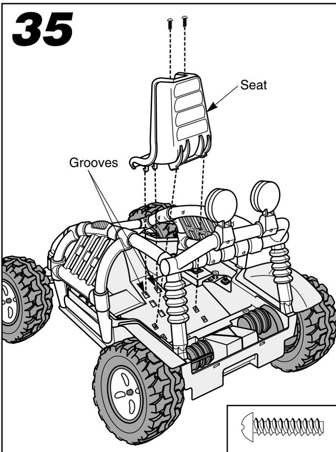
**Note:** The seat can be assembled in any one of three positions for your child's comfort.
