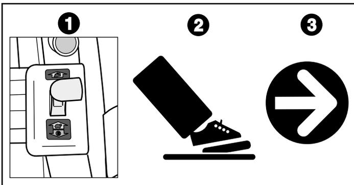
**IMPORTANT!** To avoid damaging the motors and gears, make sure to stop the vehicle before switching between low and high speeds.
