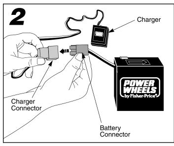
• Plug the battery connector into the charger connector. **IMPORTANT NOTE!** If you are recharging your battery, you will first need to disconnect the battery connector from the motor harness connector under the seat of your vehicle.
