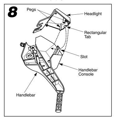
Fit the rectangular tab on the back of the headlight into the slot at the back of the handlebar console. Make sure the pegs in the top corners of the headlight fit into the handlebar console.
