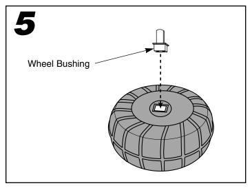
• Fit a wheel bushing into the rectangular opening in each front wheel.
