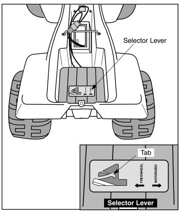
When detached from the base, your **Rock & Roll** is ready for freewheeling or motorized driving use. (See Removing Your Vehicle from the Base on page 22.). Select the freewheeling mode for some freewheeling fun:
