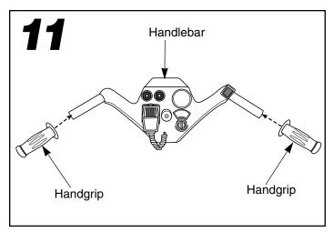
• Fit a handgrip onto each end of the handlebar.
