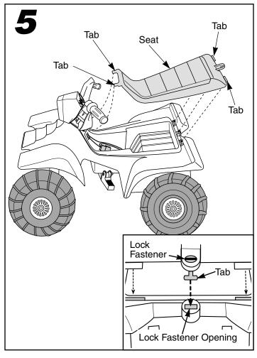
Insert the tabs on the front of the seat into the slots in the vehicle body.
