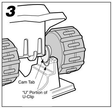
Push the vehicle forward slightly to engage the t-slider in the slot on the base. (The t-slider is on the underside of the vehicle.) The cam tabs should now be directly above the "U" portion of the U-clips.
