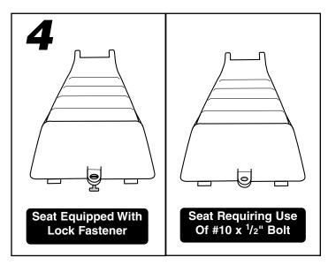
• Determine whether the seat on your vehicle is equipped with a lock fastener or requires use of the #10 x 1/2" bolt, found in the Small Parts bag, to lock the seat. If your vehicle seat is equipped with a lock fastener, please properly dispose of the #10 x 1/2" bolt.
