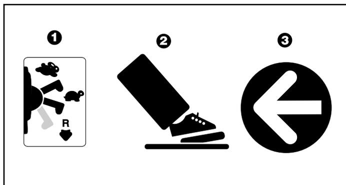
**IMPORTANT: To avoid damaging the motors and gears, stop the vehicle before shifting from forward to reverse
