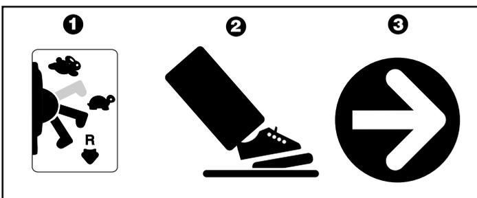
**IMPORTANT!** To avoid damaging the motors and gears, stop the vehicle before shifting between low and high speed.
